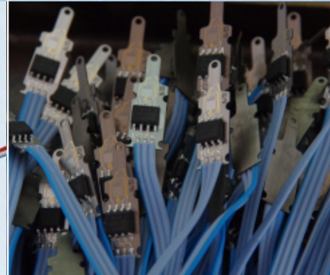
Series product for pressure monitoring and fault detection in peristaltic infusion pumps
