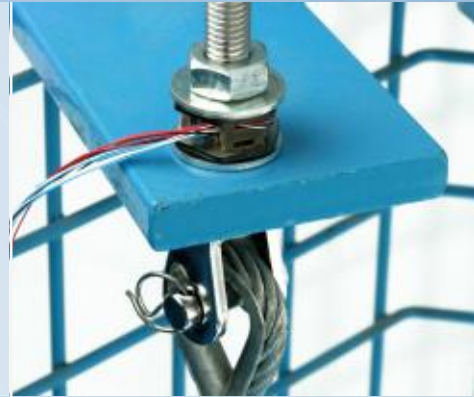
Prototype setup for a customized tension sensor consisting of standard measuring elements
