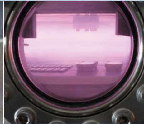
View into a sputtering system: application of thin insulation and metal layers in argon plasma
