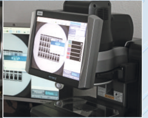
Measuring projector for efficient inspection of the geometry of sensor substrates in series production
